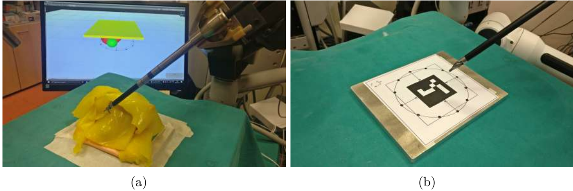
Fig. 8.2 (a) In our setup the PSM interacts with silicone fat tissue covering a kidney phantom. The simulated scene controlling PSM movements within UnityFlexML can be seen in the background. (b) The calibration board used to uniquely map all the components of our real experimental setup to the UnityFlexML environment.
